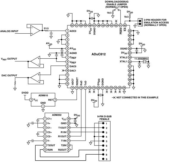
Figure 46. Typical System Configuration
